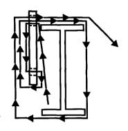
Thread sufficient length of frame tie strap through buckle as shown.
