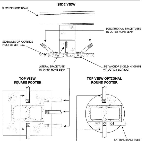
Conventional footings must be placed below frost line depth for the site unless an insulated foundation or monolithic slab is used.
