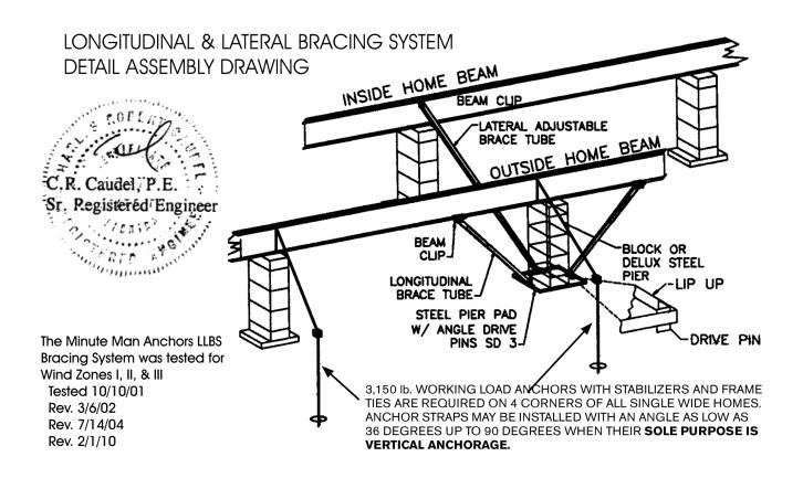
LLBS Longitudinal and Lateral Bracing System engineering certification for Wind Zones I, II & III, ground and concrete applications.
